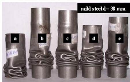
Fig. 5 Deformation modes of the collapsed mild steel specimens under various crushing types: (a) free-ends (DM); (b) biaxial-0 deg (DM); (c) biaxial-30 deg (XM); (d) biaxial-37 deg (DXM); and (e) biaxial-45 deg (DXM)
