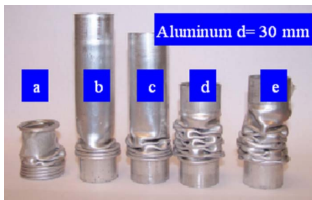
Fig. 4 Deformation modes concerning the aluminum specimens during their collapse under various loading paths: (a) free-ends (AXM); (b) biaxial-0 deg (AXM); (c) biaxial-30 deg (XM); (d) biaxial-37 deg (DM); and (e) biaxial-45 deg (DM)
